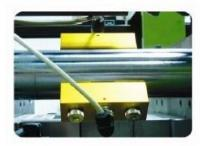
Right: 2 SML-ME on a tie bar for bending compensated measuring.
