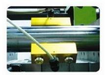
Right: 2 SML-ME on a tie bar for bending compensated measuring.
