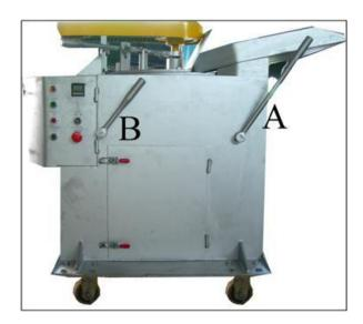
Handle "A": This Handle for closing lower cover after pouring dross out
