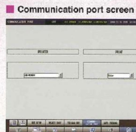
The conditions can be printed on a printer and stored on USB memory.
