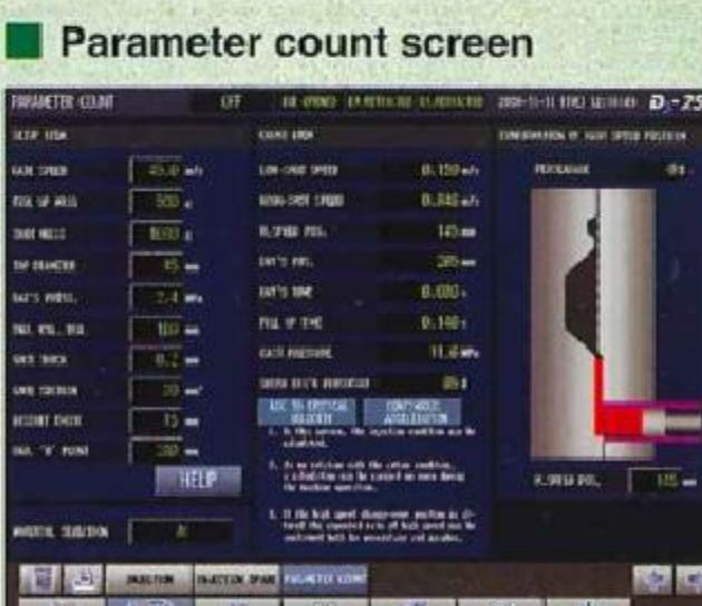
Calculates the injection parameters. The results can be checked visually.
