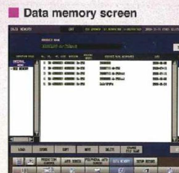
Stores casting conditions for 400 dies and graphic data for 40 dies in memory.
